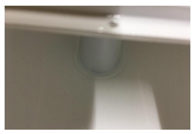
This photo taken through the main hatch clearly shows a 5 mm x 5mm lip of moulded plastic around the base of the keel box and extends out on to the hull interior. Let's hope these additions to the new boats will stop hull cracking problems from now on.
