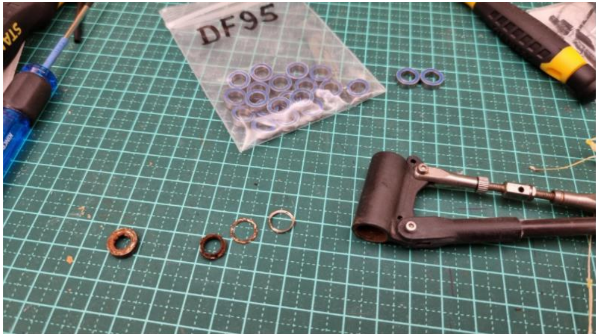
New Replacement Bearings – Stainless Steel....
