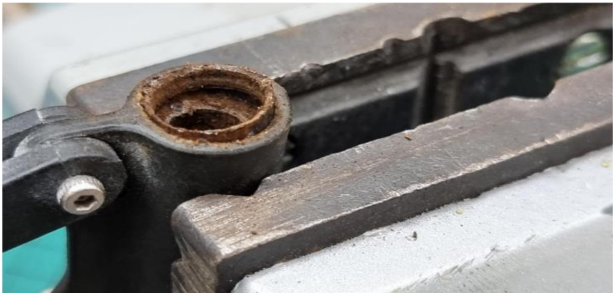
Removal of the bearing – Outer Race Case
