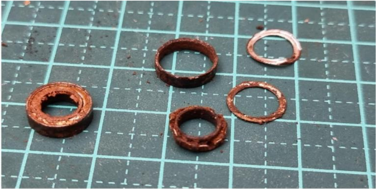
Failed / Rusted bearings removed and discarded
