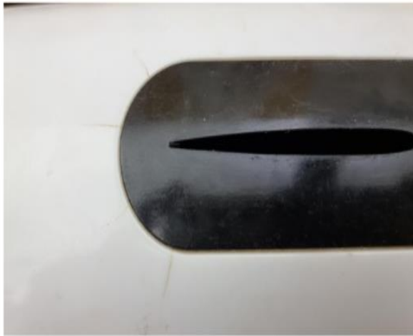
Hull Cracks visible on Hull Bottom behind the Fin Box
