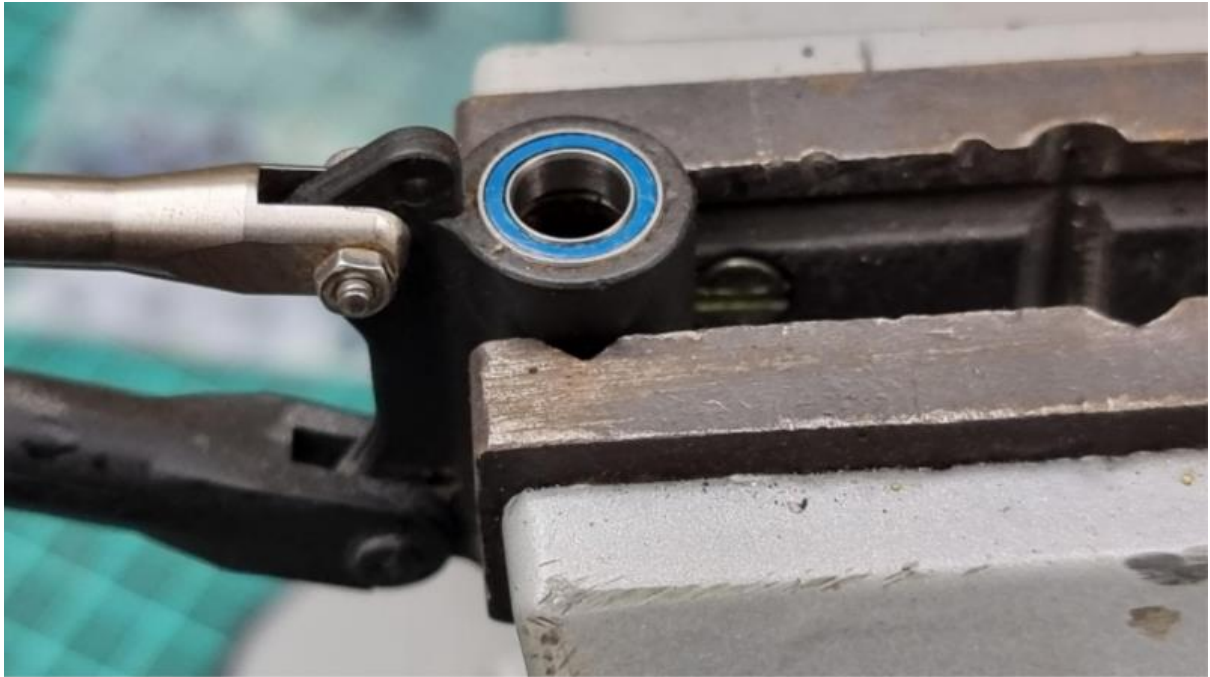
Top Boom Bearing fitment
